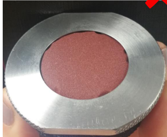
Figure 8 Example of unacceptably mounted abrasant. Creases are visible around the edge leading to an uneven testing surface.
