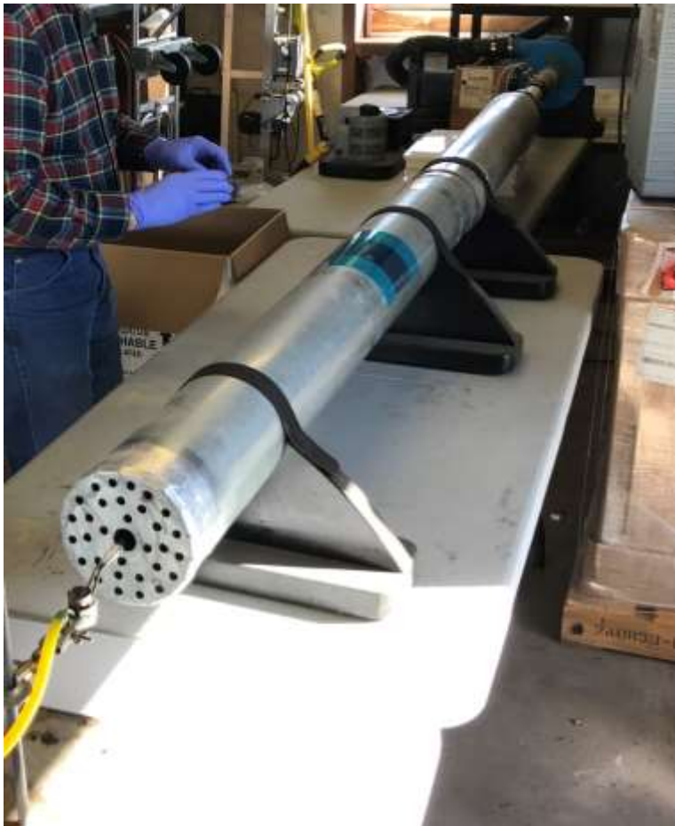
Figure 4 Wind tunnel configuration, showing the twin fluid gravity fed venturi nozzle, the baffled opening for air straightening, opening downwind from the point of atomization and at the rear an extraction fan.
