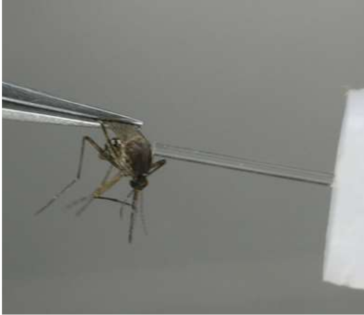
Figure 3 The dose of 0.1 \mu\text{l} being placed directly onto the pronotum of a mosquito using a capillary action micro pipette
