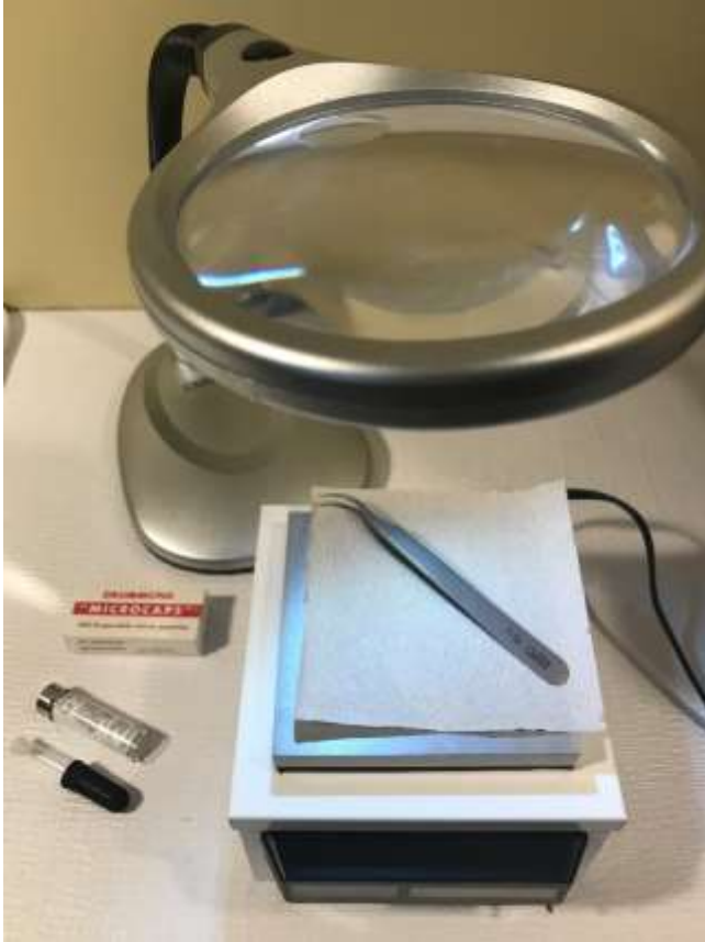
Figure 1 The chill table with magnifying light paper towel to stop condensation and prevent contamination of the table top, the micro pipettes and forceps for application of the compound and manipulation of the test mosquitoes
